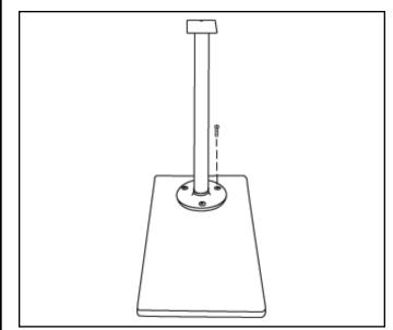
Figure 7. Securing the pedestal to the foot plate
