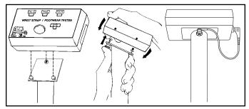
Figure 8. Installing the Combo Tester to the pedestal
