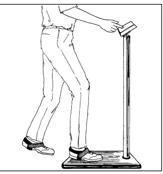
Figure 11. Performing a footwear test with the <u>770031</u> Combo Tester with Stand and Foot Plate
