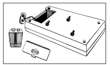
Figure 12. Replacing the battery
