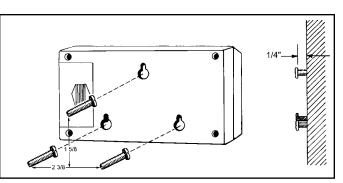
Figure 5. Combo Tester keyhole slots
