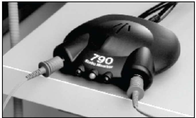
Figure 7. SCS Static Monitor 790 attached to equipment chassis.
