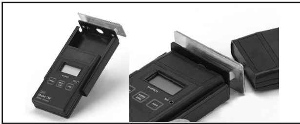
Figure 6. 718 Static Sensor charging plate in use.
