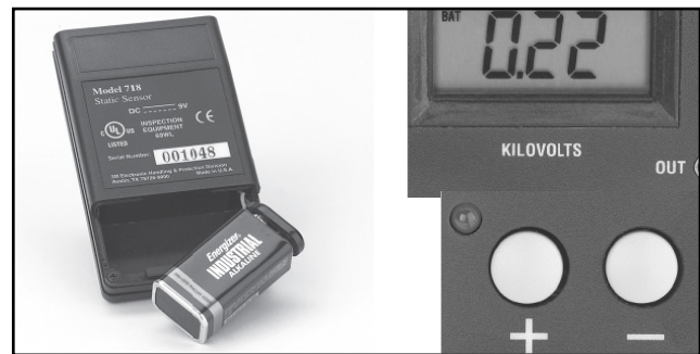
Figure 2. SCS 718 and 718A Battery Replacement and Indicators.
