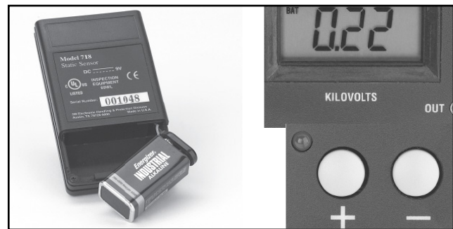
Figure 2. SCS 718 and 718A Battery Replacement and Indicators.
